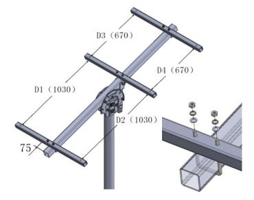
2) Preassemble the Cross Connection Clamp at the Rectangular Tube-Master with M8\*70 hex bolts, plain washer 8, spring washer 8, and M8 nut as shown in the figure below.
