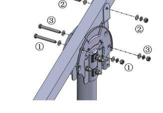
4) Fasten the Steel Cap Assembly to Pipe with M14\*150, M14\*110 Hex Bolt, keep the Rectangular Tube-Master parallel to the south-north by adjust the Steel Cap Assembly.
